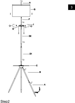
Screw the Pipe (F)onto the Socket (E),
