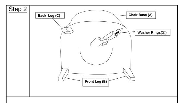
Install the Leg(B&C) into the bottom of the Chair Base (A) by placing the Washer Ring (1) onto the threaded stem.
