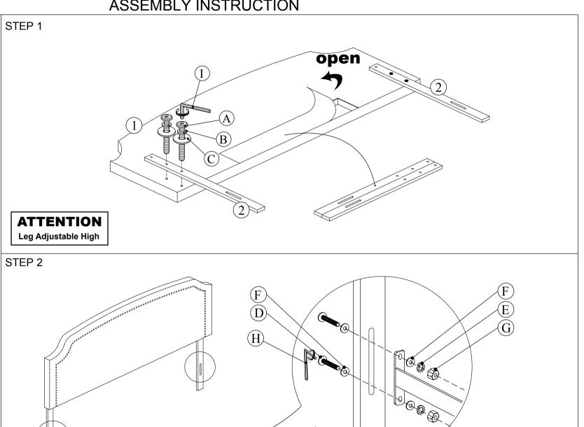
NOTE: AFTER A FEW DAYS OF ASSEMBLY, IT WILL HAVE ACCLIMATIZED TO THE ENVIRONMENT. PLEASE TIGHTEN ALL HARDWARE. CHECK TIGHTNESS OF ALL SCREWS EVERY 6-8 WEEKS.
