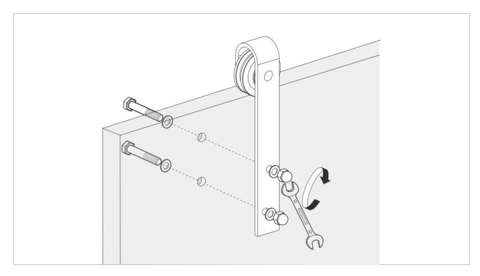
Next, position each anti-jump bumper at least 2" in from the edge of the straps. Tighten slightly to secure in place
