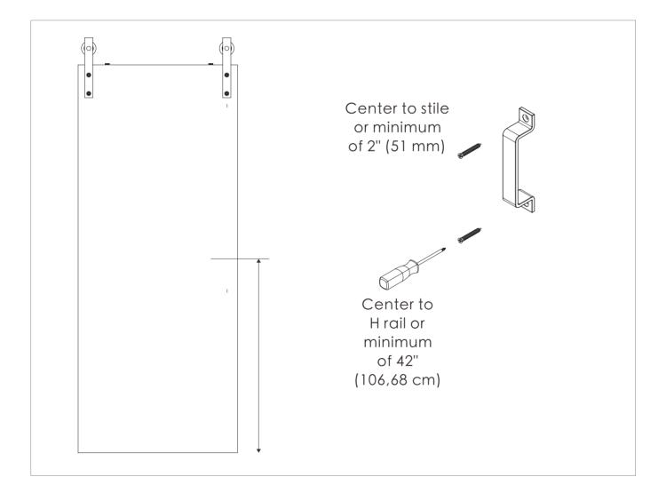
Note: using an electric powered drill to secure screws may damage the screw and door.
