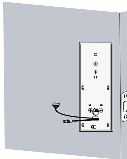
(2). Run the wires through the back cover.
