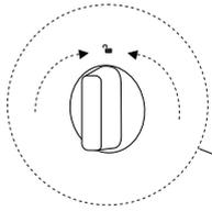
Notes: Make sure to rotate Thumbturn to the unlocked position before installing.
