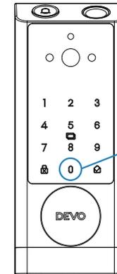
The "0" key blinks when the distribution network is activated. (Networking effective time: 120S)
