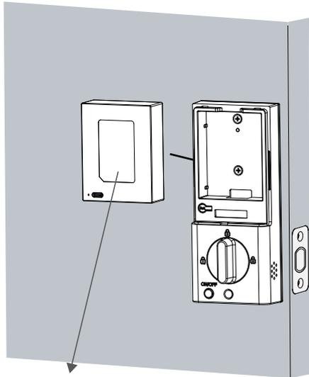
Notes: After fully charged, install the battery into the door lock and it can be used
