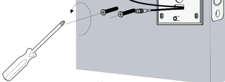
(3). Secure the back cover with screws.
