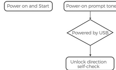
The smart lock self-checks the unlock ing direction when powered on. After the self-check is completed, the lock will be closed.
