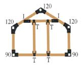
Please note: When assembling make sure brackets are facing the directions shown in this diagram.
