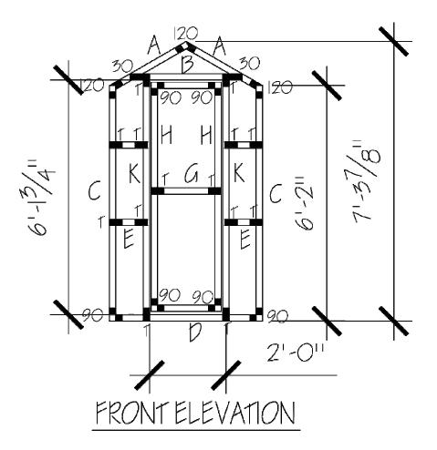
**Step 9:** Finally – measure your structure to determine the amount of materials you will need to purchase to cover your structure. Always make sure you allow for seams or waste material and purchase extra. To determine the amount of material needed for the front and rear of the structure measure the base for your width and then measure from the base to the top of the ridge for your height.
