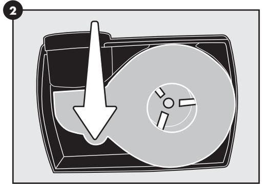
3. Use a fingernail to pull out the impeller, which is held in place magnetically. Clean the pump parts with warm water and soap, then reassemble the impeller, stator and faceplate.
