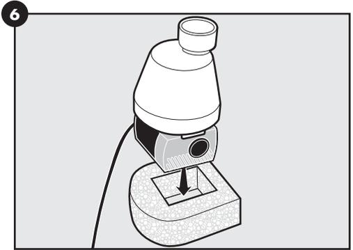
7. Place the assembled pump, filter housing and foam filter into the bottom of the bowl as shown. Press down to engage the suction cups. **Note:** Wetting the suction cups will ease assembly.
