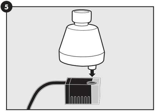
6. Place the assembled pump and filter housing into the foam filter with the cord running above it.
