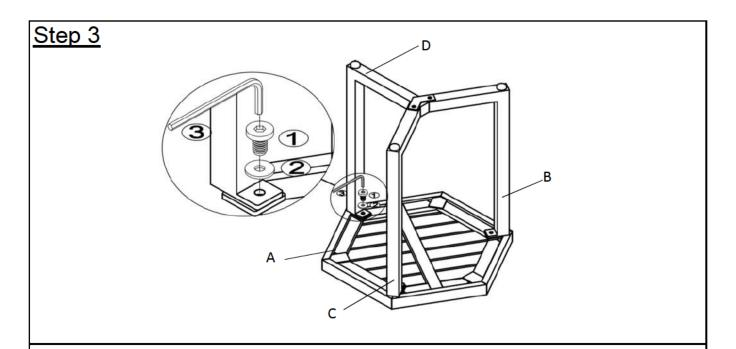
Attach the Third Leg Frame(D) to the Table Top(A) using a Bolt(1), Washer(2) and the Allen Key(3) as shown in above picture.
