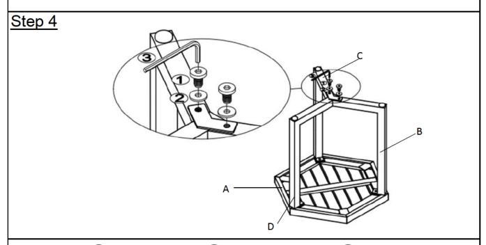
Using 2 Bolts(1) and 2 Washers(2), with the Allen Key(3), connect the Third Leg Frame(D) to the First Leg Frame(B) and the Second Leg Frame(C) as pictured.
