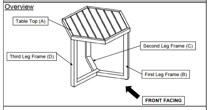
This Table has multiple parts and may require up to 10 minutes to assemble. To give you an overview of the Table parts, the above picture is to help you put the various parts into perspective. Please read through the instructions below to familiarise yourself with the parts and steps before assembly.
