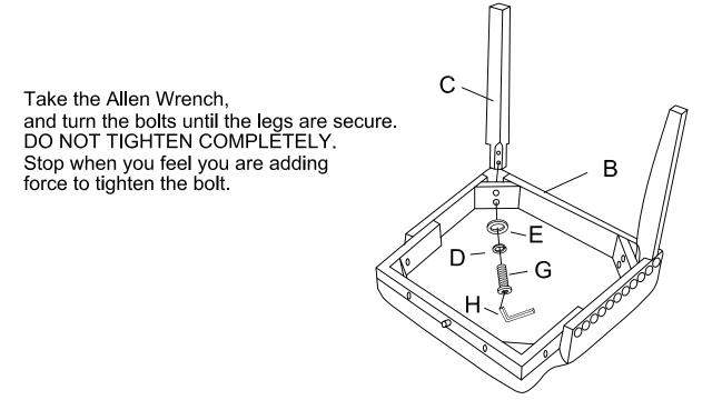
Use the bolt (G), lock washer (D), flat washer (E) in both of hole of seat (B) and chair back (A), turn the allen wrench (H) to tighten the bolt (G). But not too tight.
