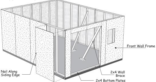
5. Unscrew and remove the 2x4 door spacer (this will be used later). Cut and remove the bottom 2x4 in the door opening.
