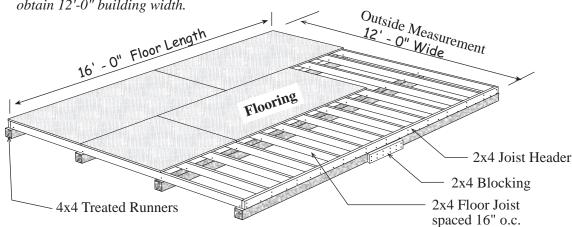
It is important that the floor be level and square. Square the floor as follows: before nailing the flooring, measure the floor diagonally (corner to corner). Then measure the opposite corners; these measurements will be the same when the floor is square. Toenail frame to the 4x4 runners.
