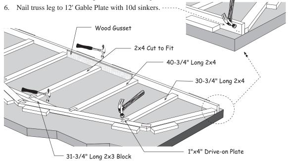
7. Position 2nd gable plate and repeat steps to assemble the front roof gable. Read note below:
