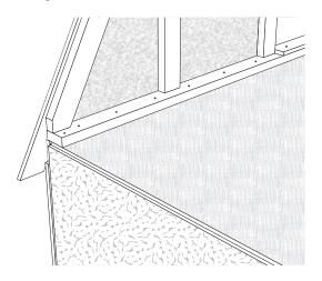
1. Install the rear gable on the rear wall. The siding on the gable must extend over the 1x4 trim board, not behind it. See detail 'D' below. Nail bottom gable to loft flooring. Use 10d sinker nails spaced evenly in stud openings.
