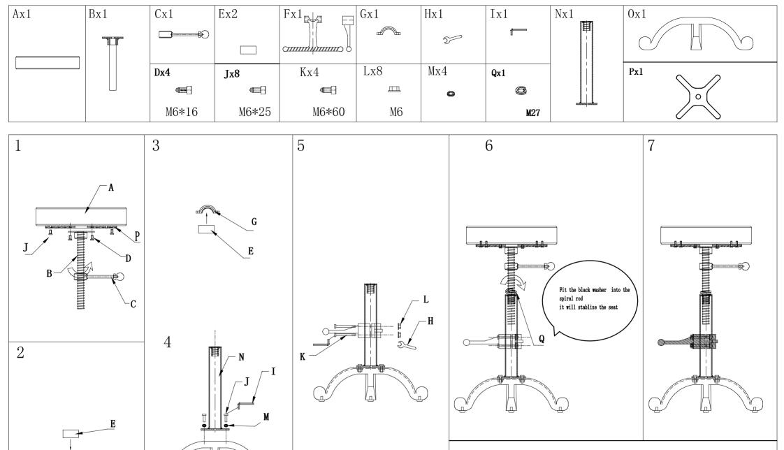
Part D and J,The screws need to be screwed at the same time, then locked with a wrench.
