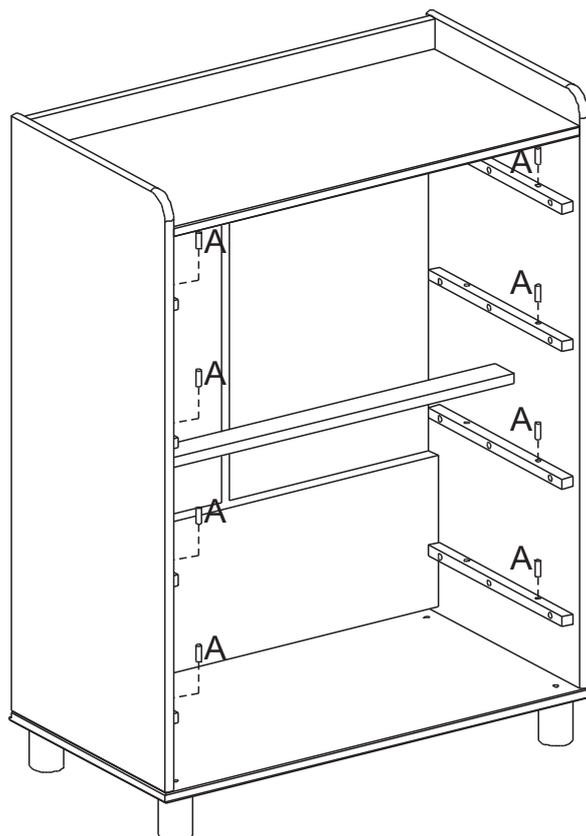
Insert wood dowel (A) into part (8) (Runner small).
