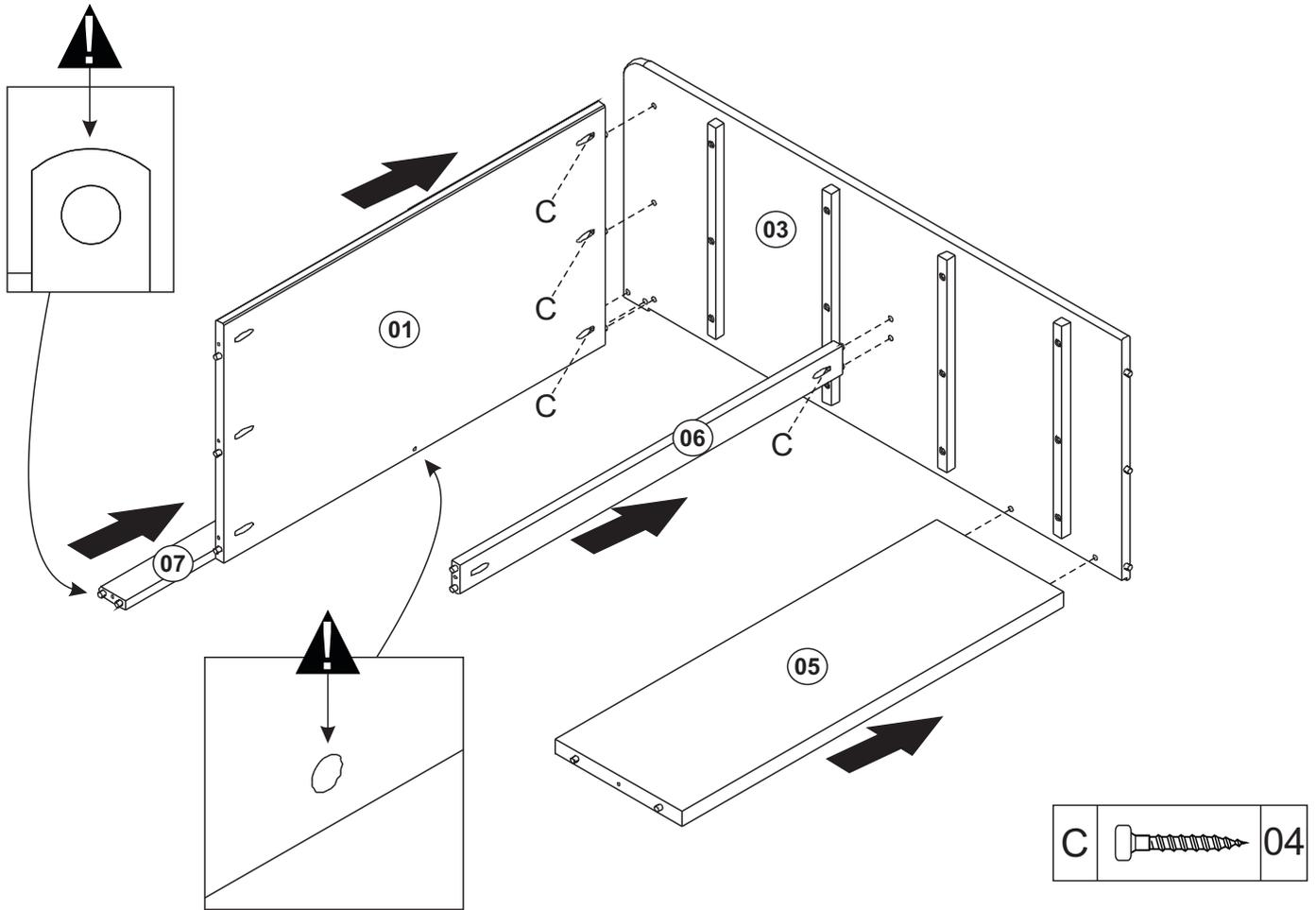
Step 4 Insert screw C (x4) into parts (01),(06).
