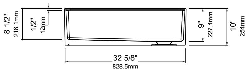
**NOTE:** Due to the typical  $\pm 3$ mm side wall variance in manufacturing, it is recommended that you design / modify the sink cabinet to match your clients individual sink(s) need.
