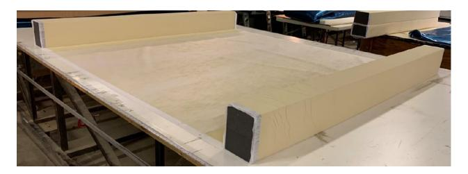
The set of Yellow or Blue Fabric Covered Foam **Side Rails** should be unrolled and laid out next. Place over top of the Head/Foot Rail fabric. One Foam Piece should be on each side of your wood decking and sitting <u>IN BETWEEN</u> the **Head and Foot Rails** as shown in the reference image below.
