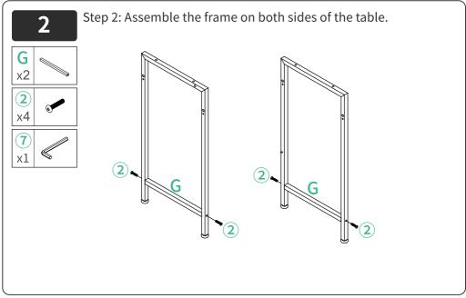
the figure. Note: Too tight screw ② may cause cracking of the table board. х1 х1 х1
