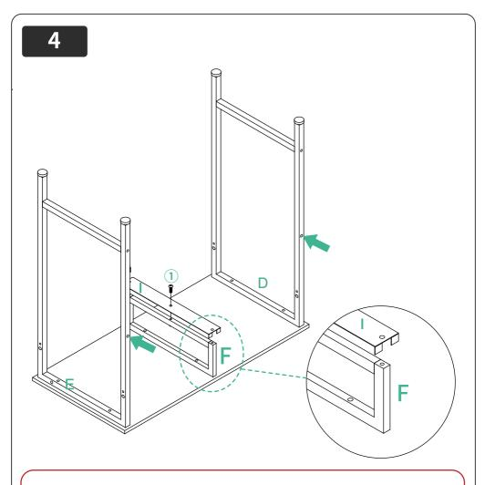
Note: During installation, make sure that the two stop plate of Part I are on the same side as the holes on parts E and D in the figure.
