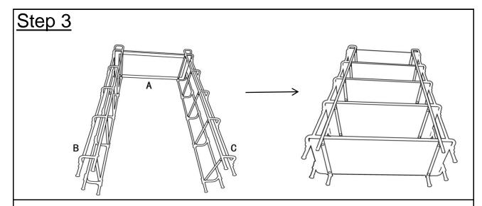
Repeat Steps 1 & 2 with remaining 4 Wooden Shelves(A) from top to bottom. At this stage, loosely tighten.
