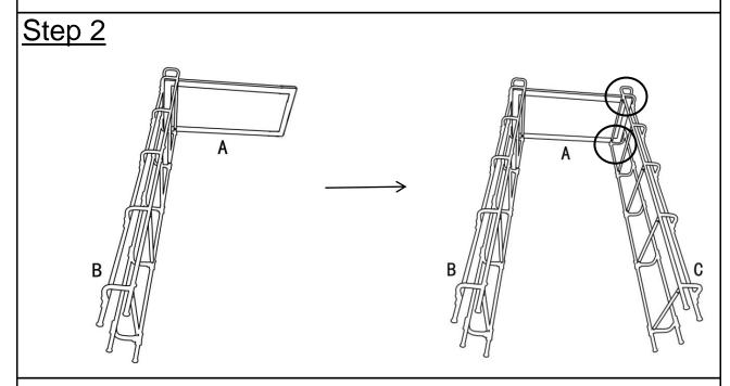
Attach Wooden Shelf(A) to Right Leg Frame(C) using Bolt(3) with Allen Key(4). At this stage, **loosely tighten.**
