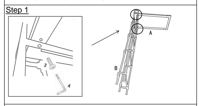
Open the carton and place all parts onto a clean, non-marring surface. Place the Left Leg Frame(B) on it's side as shown.
