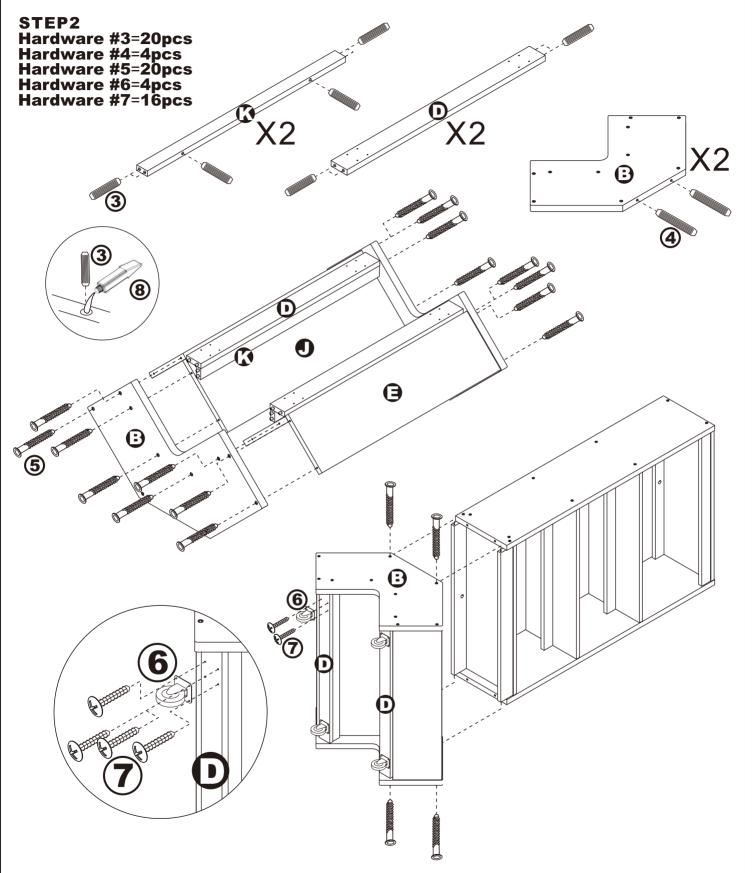
Make sure the product is rested on a flat surface and does not feel loose or wobbly. If it does, double check that the bolts/screws are secured and properly tightened.
