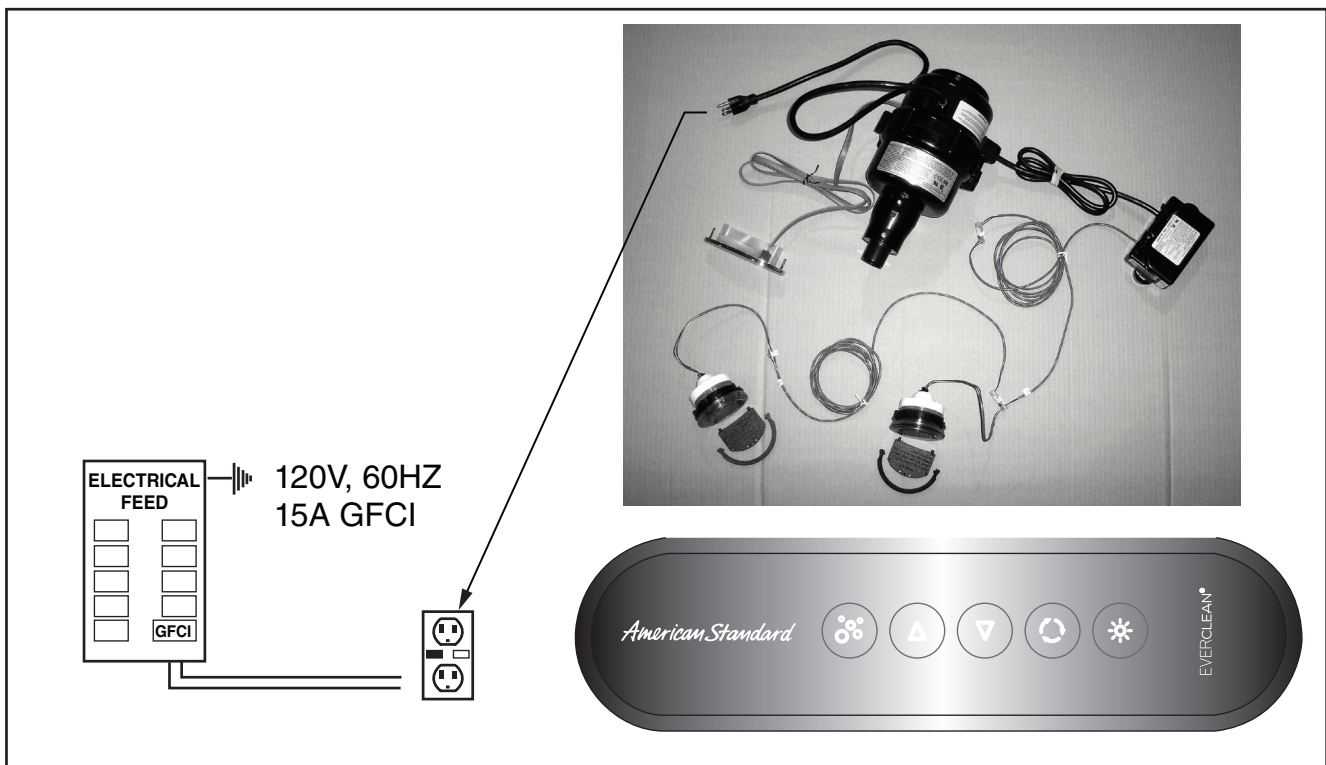
ELECTRONIC ACTIVATED AIR BATH WITH LIGHTS (5 BUTTON PANEL)
