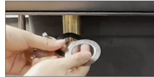
03. Separate the gaskets and screws
