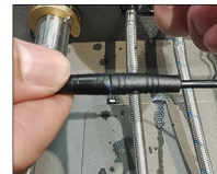
04. Connect the electricity line with motor
