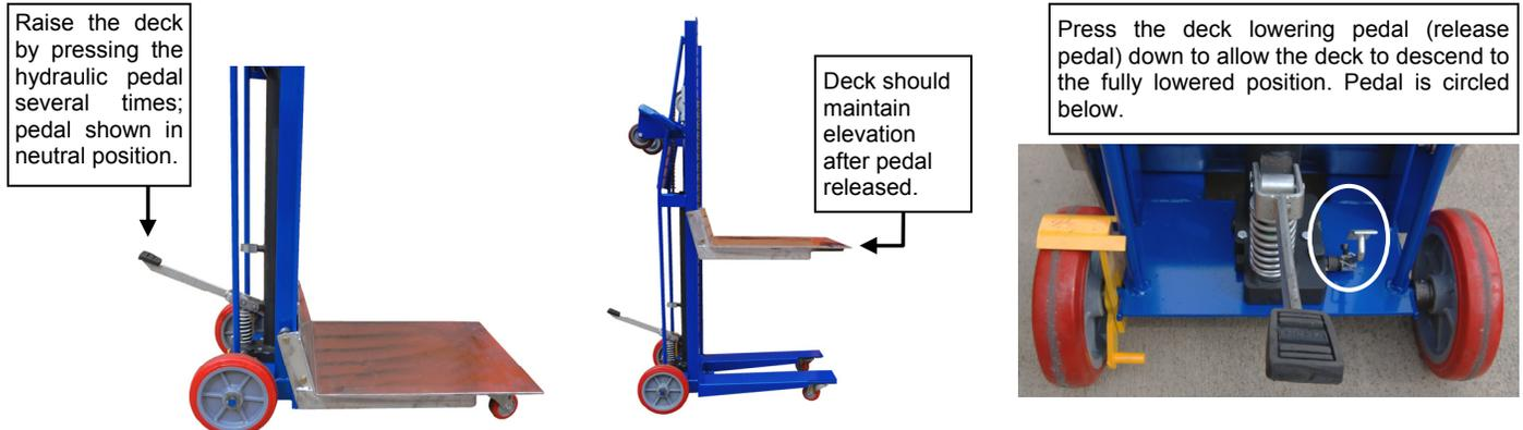
II. Wheels/Rollers: to verify that the wheels turn smoothly and are undamaged, push the lifter far enough to allow the rear wheels to complete a few full revolutions. If the lifter wobbles as you push it, check the surface of each wheel for embedded debris. Remove all debris; then repeat the process to determine whether the vibration problem has been resolved. If the problem persists, notify maintenance personnel.
