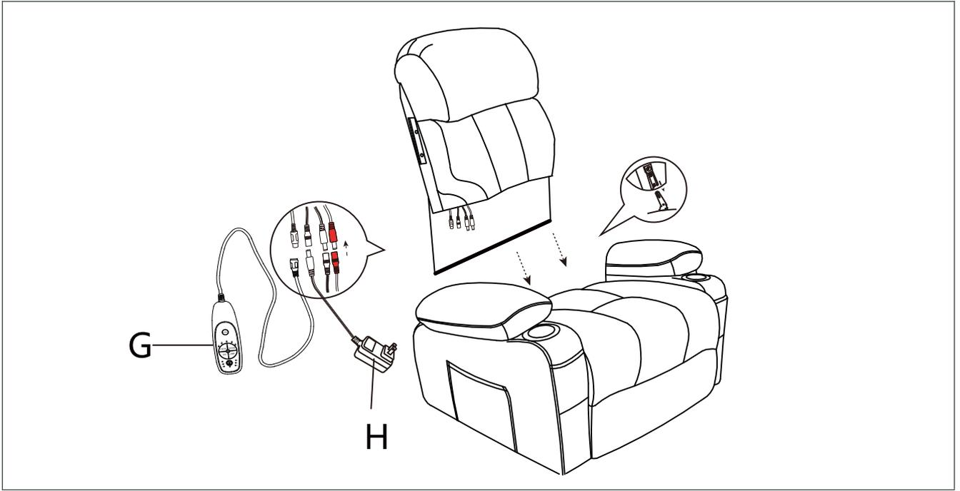
**Step10:** Insert the back ear so that it can be installed into the back side. When they engage, you will hear a "click" sound.
