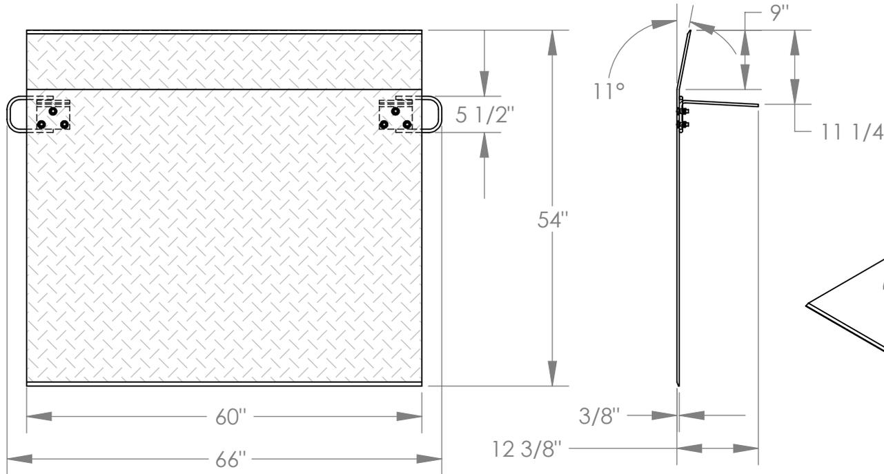
NOTE: BEND OR CROWN IS 11° AND LOCATED 9" FROM EDGE OF DOCKPLATE
