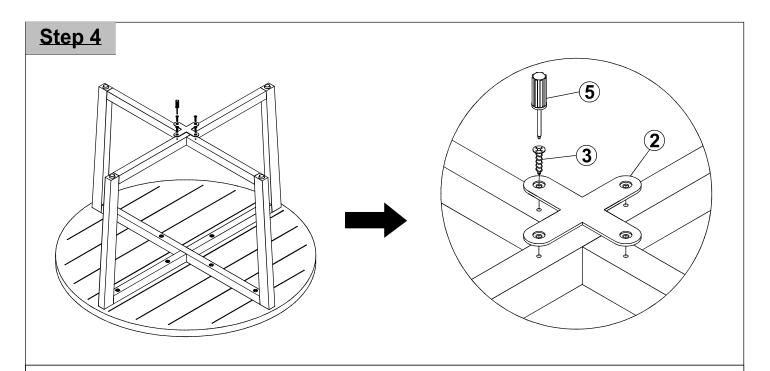
Position Cross Hinge (②) into the Cross Position of First Leg Frame (B) and Second Leg Frame (C) as picture above.
