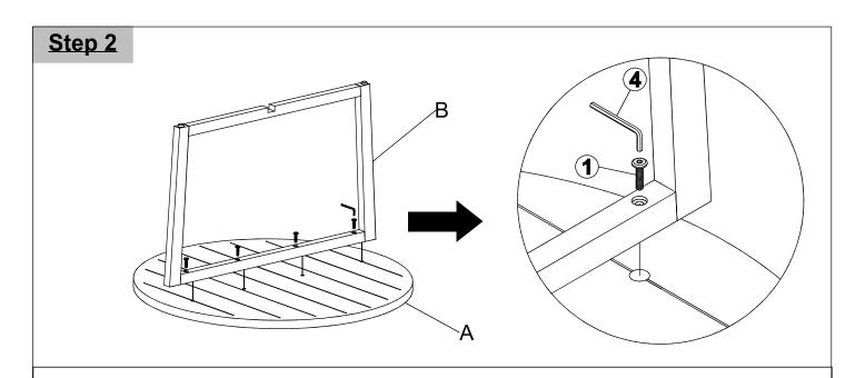
Place Table Top (A) with its underside skywards onto a clean, soft surface to avoid any scratch or damage to the product.
