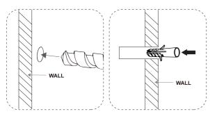
(1) Drill holes at marked (2) Press the protective location.
