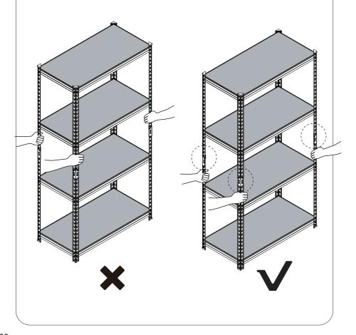
(3) For the overall stability of shelves, every cross bar (2&3) must be knocked fully tight into the end while installing.
