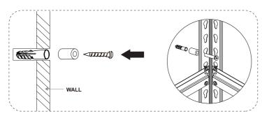
(3) Fix the safety lock on the wall with bolts.
