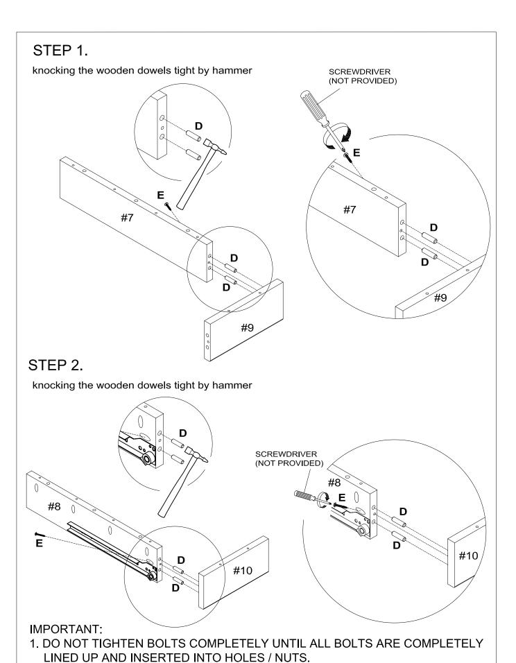
2. DO NOT OVER TIGHTEN SCREWS AND BOLTS TO AVOID STRIPPING.
