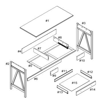
For ease of identification all parts are labeled to correspond to the Step number in which the part is used.
