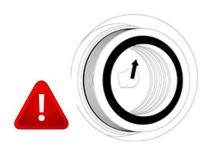
If you found the lamp won't illuminated after wire installed and inserted a E26/E27 light bulb, please try to raise up the internal metal contactor in the socket.please make sure the power was disconnected before operated.
