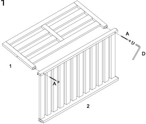
Use wrench (D) to secure seat frame (2) to back frame (1) with screw (A).
