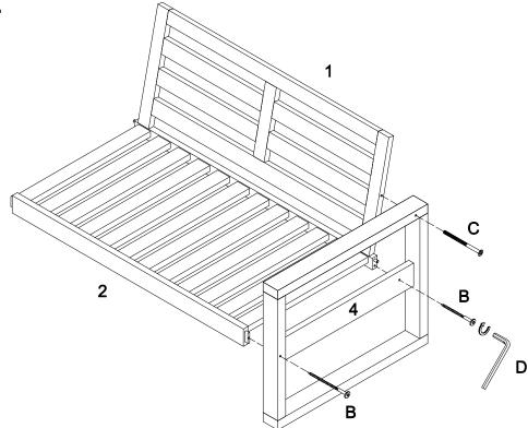
Use wrench (D) to secure side frame (4) to seat frame (2) and back frame (1) with screw (B) and bolt (C).
