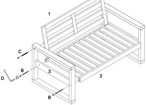
Use wrench (D) to secure side frame (3) to seat frame (2) and back frame (1) with screw (B) and bolt (C).
