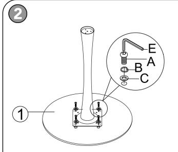
a)With assistance, lay Table-top (1) flat with the bottom-side facing up on a material that does not scratch or damage the part. b)Position Leg with Top Plate from STEP 1 as shown and align the screw holes on top Plate to screw holes on bottom side of (1). c)Use Screw (A) fitted with Spring Washer (B) and Flat Washer (C) to fasten Top Plate to Table Top.Use Allen key (C) to drive (A). Do not tighten (A) completely until all 4 screws are in place.
