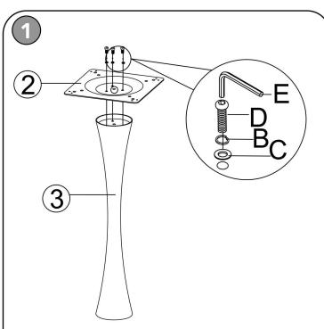
a)Position Leg (3) and Top Plate (2) as shown and align screw holes on both parts.
