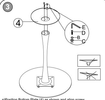
a)Position Bottom Plate (4) as shown and align screw holes on (4) to the screw holes on the leg.
