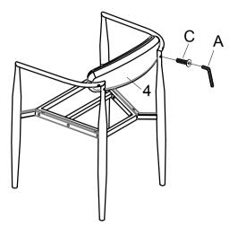
Don't lock the bolts tightly first, level the chair and tighten all the bolts at the end.
