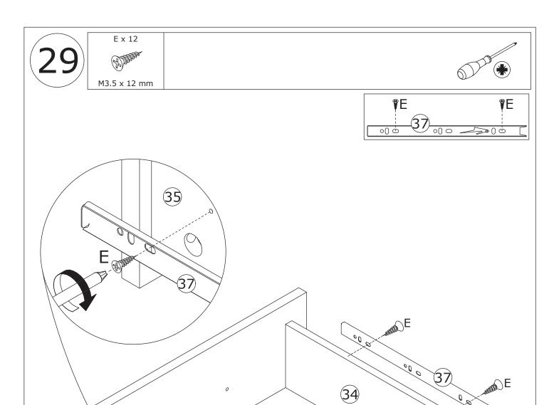
Fix track 37 to panel 34 and 35 with screw(E) as shown.
