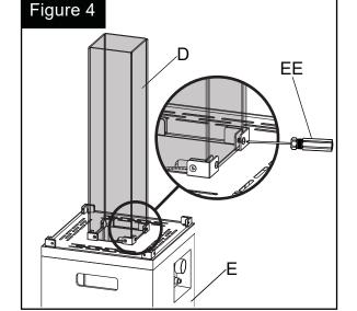
4. Cover and clamp the four narrow glass (D) with glass fixture (B) carefully. Afterwards, tighten the bolts (AA), but not tighten too much to avoid the glass pieces being damaged (See Figure 5).
