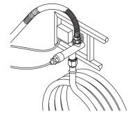
gas valve / bellows connection (Figure 13)
