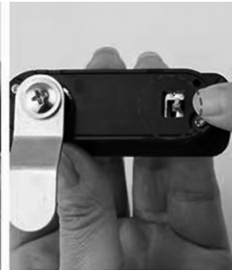
5. Reset the lever to the initial position
