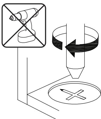
**EN**\_Turn cam lock clockwise to tighten.
