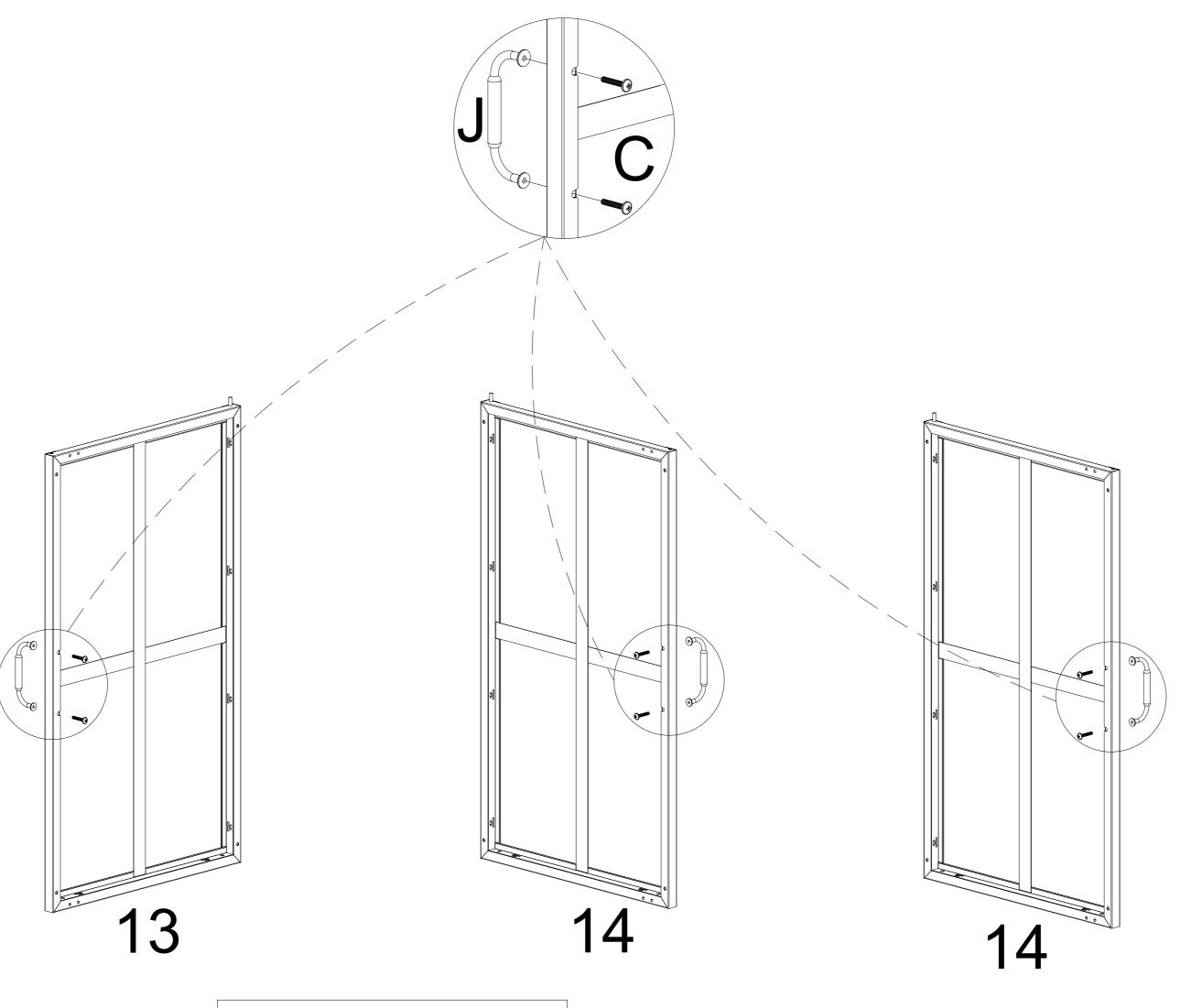
Install the handle in place according to the diagram.
