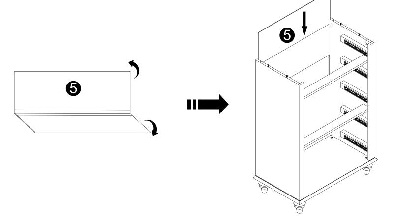
·Carefully slide panel (5) into place along the back of the assembly.
