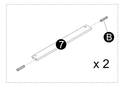
· Insert dowels (B) into panels (6,7).
