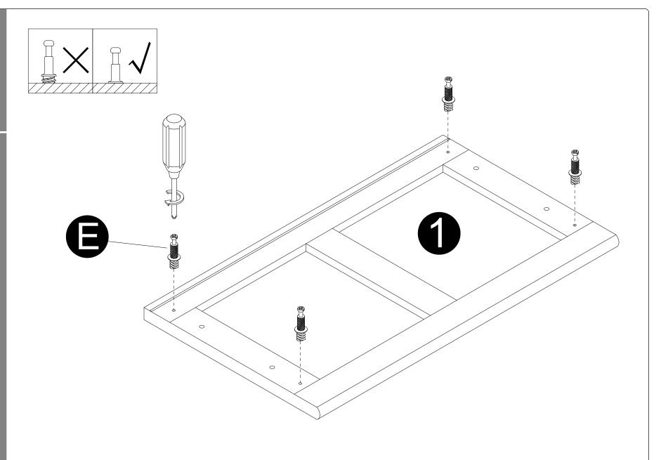
· Screw cam bolts (E) into panel (1).
