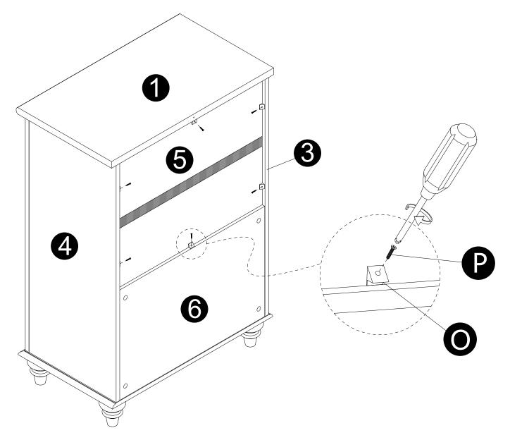
· Secure parts (O) to panels (1,3,4,6) using screws (P).
