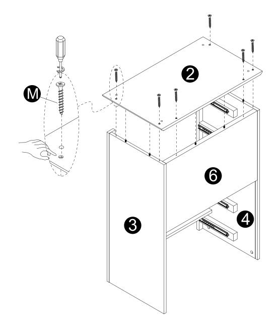
· Attach panel (2) to panels (3,4,6) using screws (M).
