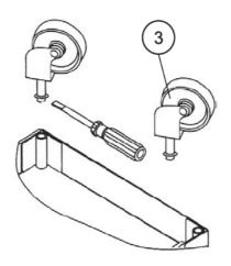
Assemble screws with a screwdriver.
