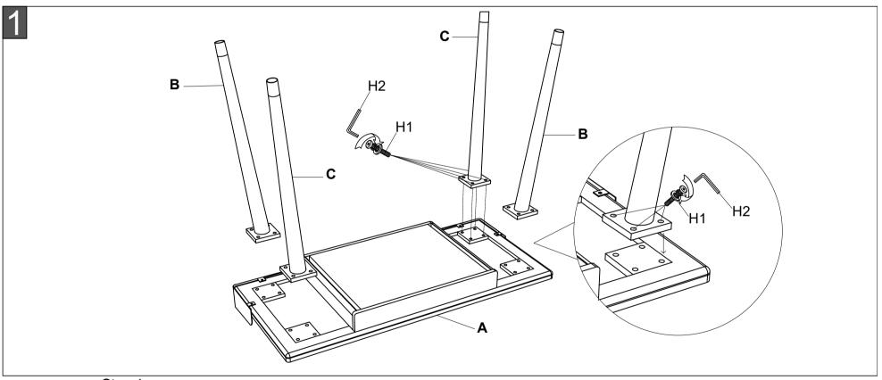
Step 1: Assembly 2\*left legs (B) to the underneath of the table top (A
