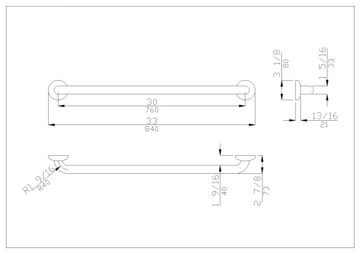
Straight grab bar, made of seamless zinc-plated steel pipe, coated with antimicrobial, biocompatible and warm-to-the-touch vinyl/PVC coated
