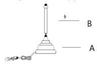
Step 3. Gently screw the rod with socket (C) into the rod (B).
