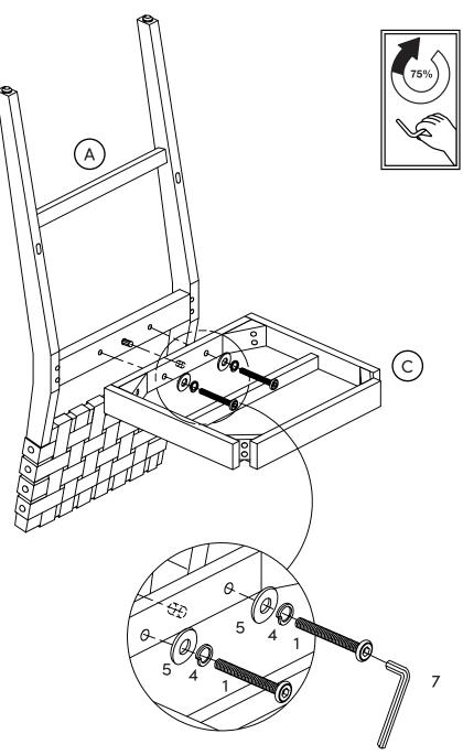
Please take a moment to match the sticker on the bottom of the chair back with the sticker on the corner block. Then, secure the Seat Frame (C) using the 1/4 x 3 1/8 inch Hex Button Head Bolt (3), Do not over-tighten hardware! 1/4 inch Lock Washer (4), and 1/4 Tighten only 75% for now. inch Flat Washer (5).
