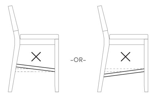
Re-check to confirm that the proper legs are installed in their intended position on the proper side of the stool.
