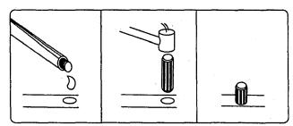
APPLY GLUE INTO PRE-DRILLED HOLE, AND GENTLY TAP WOOD DOWEL INTO THE HOLE WITH RUBBER MALLET.
