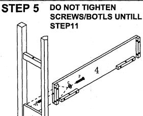
Joint the right side frame (1) and right apron (4) with bolt (F) and washer (C)
