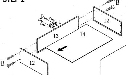
Assemble drawer plastic glide (I) to drawer backpanel (13) by using screw (J);
