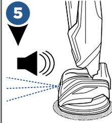
Solution will spray out of the nozzle on the front of the foot. You should hear a soft buzzing noise each time you press the SPRAY button to indicate solution being dispensed.
