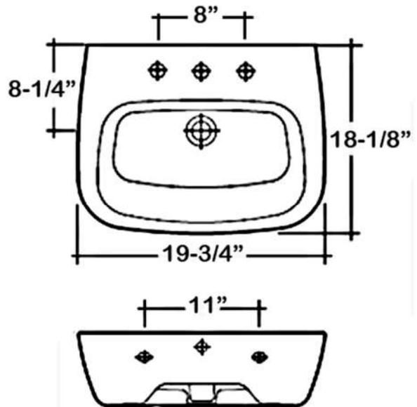
Dimensions of fixture are nominal and may vary within the range of tolerances established by ASME Standard A112.19.2.2013. Dimensions and specifications subject to change without notice.
