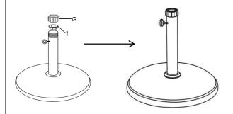
For the Umbrela Pole with diameter as 38mm, use Dia. 38mm Adapter (H) & Dia. 48mm Adapter (I) added together, insert the Dia. 48mm Adapter (I) into the Support Pole (E) first, and then put the Dia. 38mm Adapter (H) onto the Dia. 48mm Adapter(I), Turn the Cap(G) onto the Support Pole(E) to hold the
