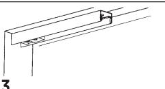
Ensure that the pivot bracket in the track is at the side which you prefer your doors to open toward. Now, fasten the track along the center line of the header, using screws provided.
