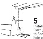
Install jamb bracket Place jamb bracket, tight to floor, so that center hole of bracket is plumb with hole in the top pivot bracket (in track).
