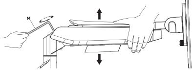
To properly balance the arm with monitor mounted, adjust the spring tension using the supplied Allen Key as follows:
