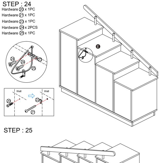
Make sure the unit is rested on a flat surface and does not feel loose or wobbly. If it does, double check all bolts/screws are secured and properly tightened.
