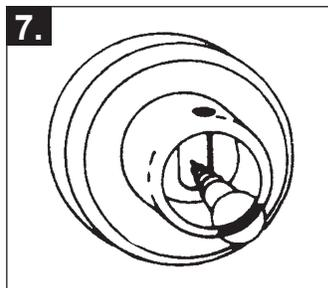
7. Secure mount to wall with screw. **Note:** Allen set screw must be at top of mount.
