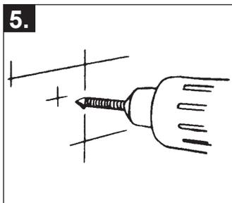
5. Drill hole for top mount. Use 1/4 inch carbide drill for ceramic tile.
