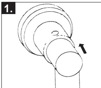
1. Place end mount of wall bar into the mount - do not tighten the set screw.
