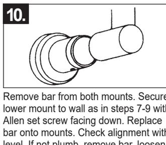
10. Remove bar from both mounts. Secure lower mount to wall as in steps 7-9 with Allen set screw facing down. Replace bar onto mounts. Check alignment with level. If not plumb, remove bar, loosen mount screws and adjust accordingly, retighten screws and replace bar.
