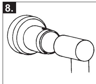
8. Place bar into mount. Do not tighten Allen set screw.
