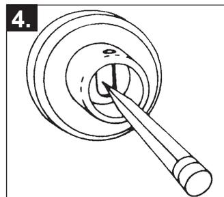
4. Remove bar mount from bar. Place in marked position on wall and mark center screw hole on wall. Do not mark lower mount at this time.
