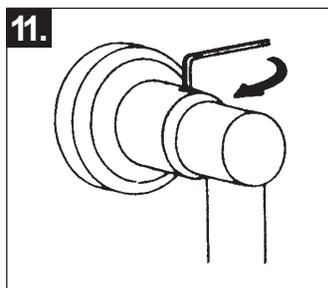
11. Tighten Allen set screw on both top and bottom mounts.
