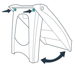
Unfold the steps by pulling back on the leg until the locking tabs snap into place. Attach the adhesive-backed fabric treads and feet.
