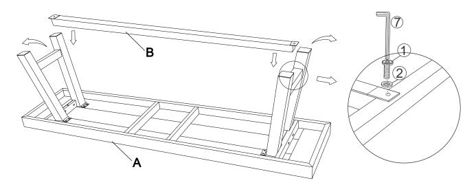
Attach the Leg Connector (B) to the Bench (A), You may need to apply a little pressure to the Bench Legs - pushing outwards to position the Leg Conector (B).
